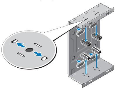
**2** Mount the wall-mount unit to the wall using the screws that shipped with the unit.
